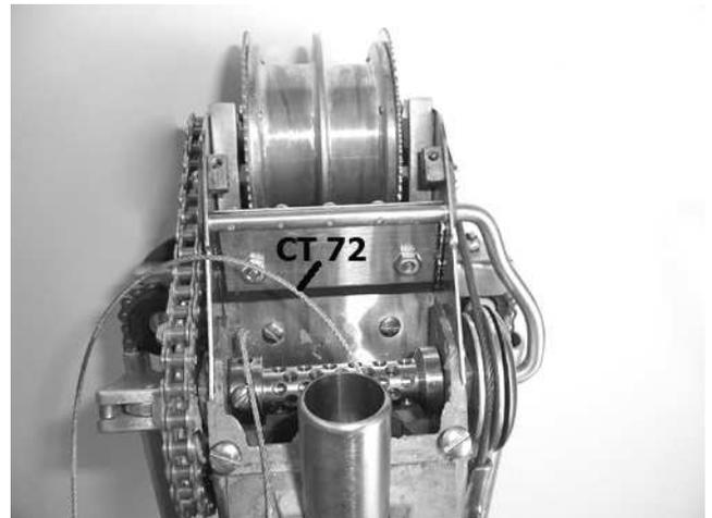
4) Remove three screws that hold guard ring on end of taper tube.
