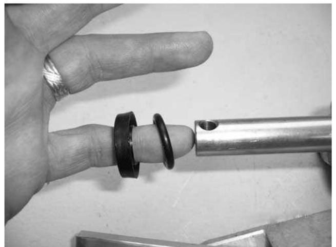
19) Slide seal and o-ring over shaft.
