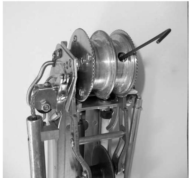
3) Drive drum and shaft removed.
