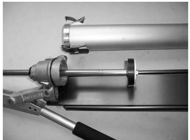
4) Cylinder and piston shaft off.
