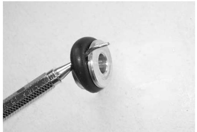
16) New o-ring prior to installing on wheel.
