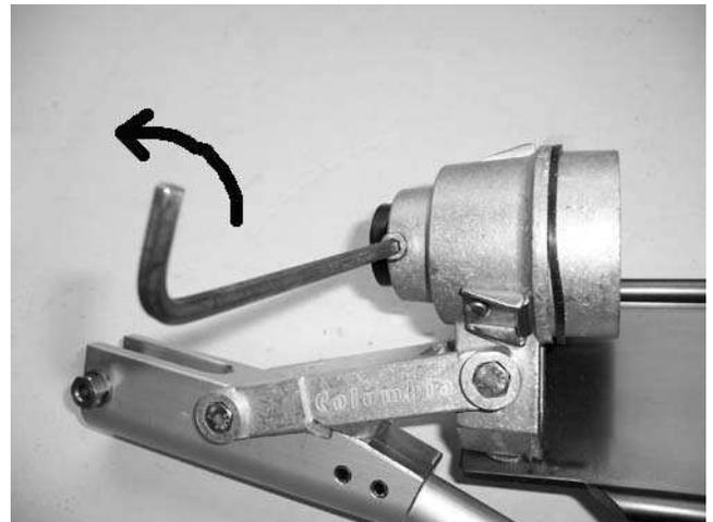
6) Bushing (MP 5), seal (MP 23) and o-ring (MP 23A) off. *\*\*Note order of parts when re-assembling.*
